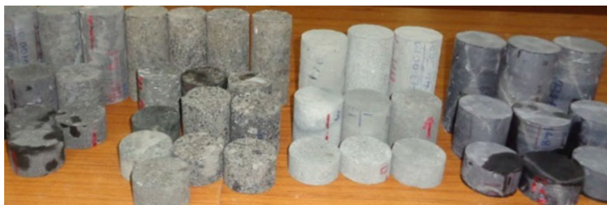
Fig. 2 Specimen prepared for testing under tensile, uniaxial, and triaxial loading
