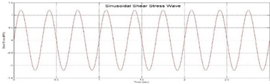
Fig. 3 Input sinusoidal shear stress waveform at the base of the model
