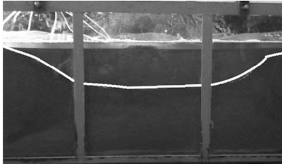
Final Failure - Reinforcement at Base of Embankment
